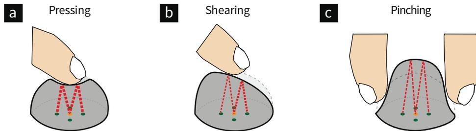
Fig. 4. Deformation sensing using four light diodes: (a) pressure deformation increases the amount of measured light on all diodes; (b) shear deformations change the amount of measured light asymmetrically; (c) pinch deformations decrease the amount of measured light on all diodes.
