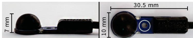
Fig. 5. Sensor used in our prototypes.
