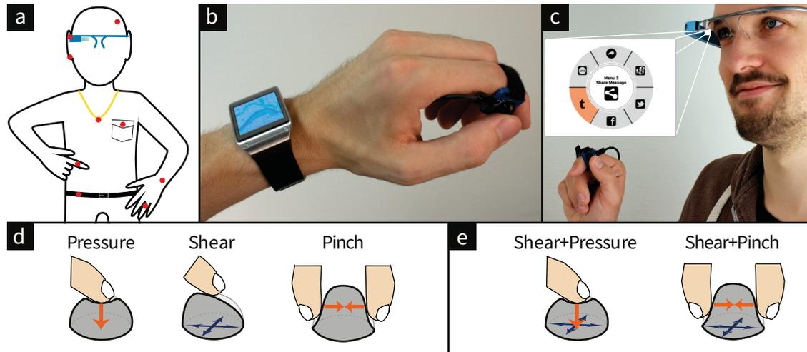
Fig. 1. (a) DeformWear enables expressive deformation-based input on various body locations: (b) One-handed input for smartwatches; (c) discreet input for head-mounted displays; (d) deformation primitives, and (e) their fluid combinations.
