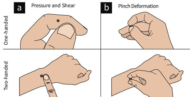
Fig. 3. DeformWear supports one-handed and two-handed input: (a) pressure and shear deformations; (b) pinch deformations.
